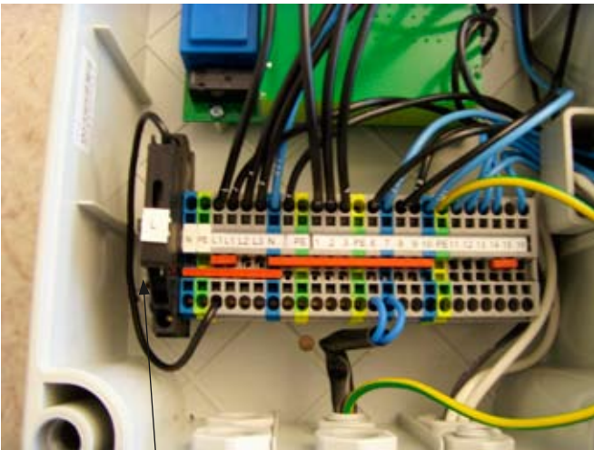
Fit an end stop as shown in the image.
