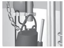
Fig. 12 Chain fitted to pump
