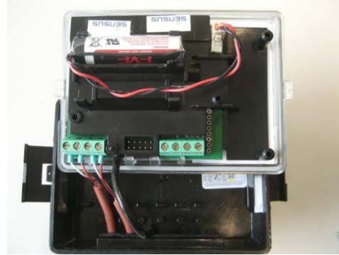
Fig. 5: Example of temperature sensor connection
