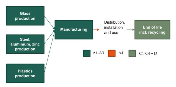
Tempered glass, steel, aluminium, zinc and plastics (polyamide, polyvinylchloride, acrylonitrile butadiene styrene, ethyl acrylic acid) are transported to a manufacturing plant where shower enclosures are manufactured. The shower enclosures are transported to a central warehouse, where they are distributed to the final customers. After use the product is transported to waste processing, is manually disassembled, and different materials are treated in their respective way.
