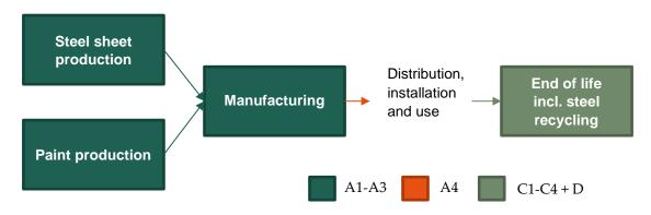
Steel sheet and paint (powder coating) are transported to a manufacturing plant where the radiators are manufactured. The radiators are transported to a central warehouse from where they are distributed to the final costumers. After use the product is transported to waste processing, and the steel is recycled.
