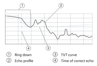
Ring down times that extend past the near range area can be interpreted by the device as the material level and are characterized by a steady high level being reported.
