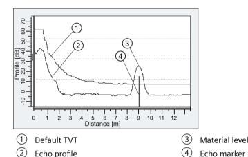
A TVT hovers above the echo profile to screen out unwanted reflections (false echoes). In most cases, the material echo is the only one which rises above the default TVT. In a vessel with obstructions, a false echo may occur. For more information, see Auto false echo suppression and Custom TVT (Page 194).
