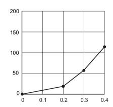
This calculation creates a piece-wise linear approximation of the level/flow curve, providing best results if the curve is non-linear and there are no sharp angles.
