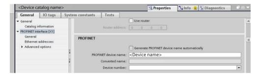
Ensure that the device name matches the device name set in your PROFINET I/O controller or the device will not establish communication with the I/O controller.
