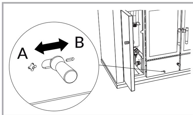
Picture 37 - Auxiliary regulation of the primary air: the valve is open at the position indicated with the letter A, while it is closed at the position indicated with the letter B.
