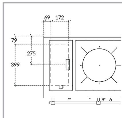
Picture 12 – Position of the lower hole for the passage of the air intake conduct. Dimensions in mm.
