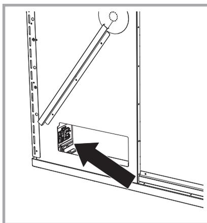
Picture 14 – Position of the terminal board for the connection to the network.
