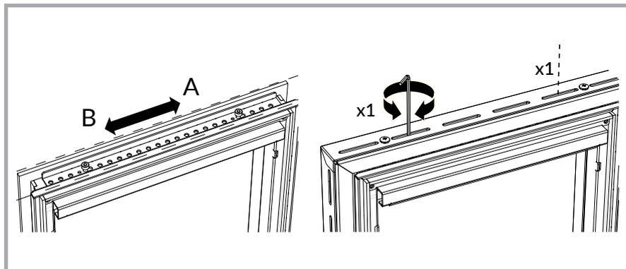
Picture 40 - Auxiliary air adjustment for glass cleaning: the plate is open at the position indicated with the letter A, while it is closed at the position indicated with the letter B.
