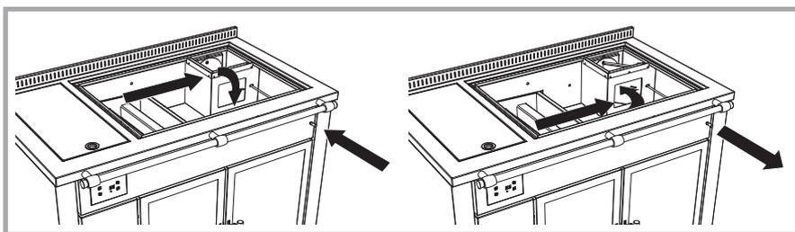
Picture 35 – Starting key. With open lever the key is open to make the starting easier. With closed key the thermal cooker is set for normal working.
