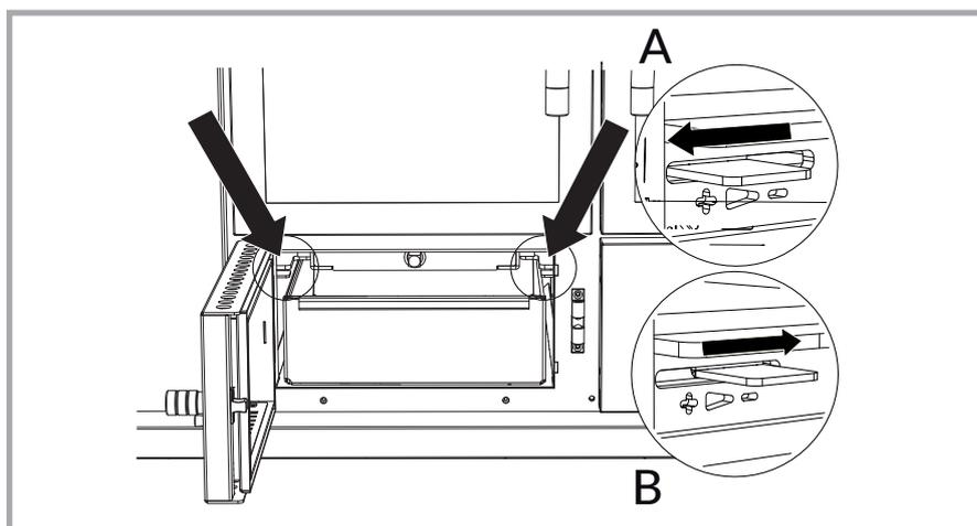
Picture 38. Secondary air regulation: the regulation is open in correspondence of the position indicated with letter A (bigger inflow of secondary air than primary air), while it is closed in correspondence of the position indicated with letter B (bigger inflow of primary air than secondary air).
