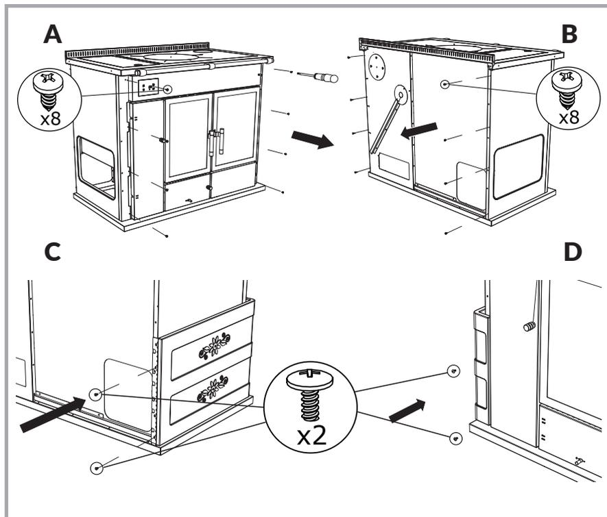
Picture 13 – Position of the screws on the device to fix the covering of the sides and fixing of the sides covering elements.
