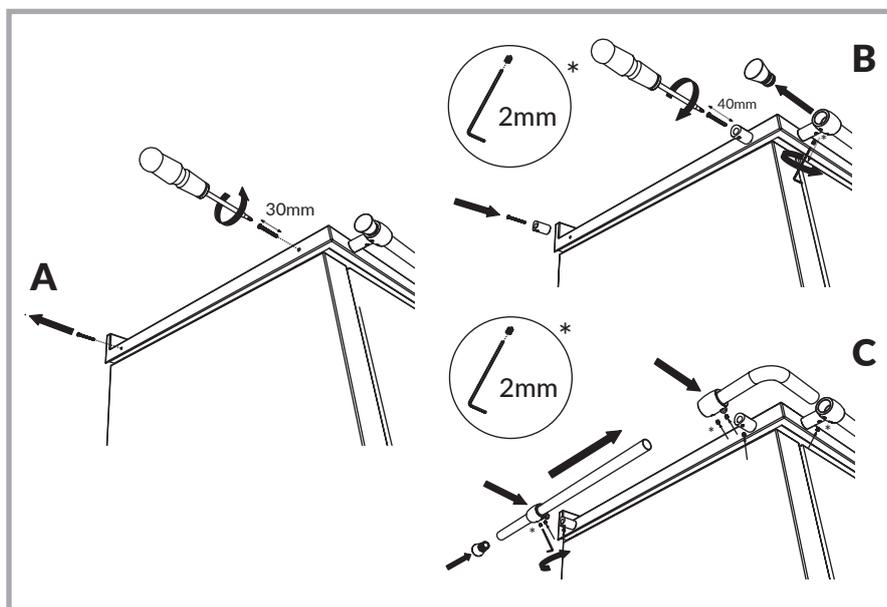
Picture 16 - Modification of the handrail.
