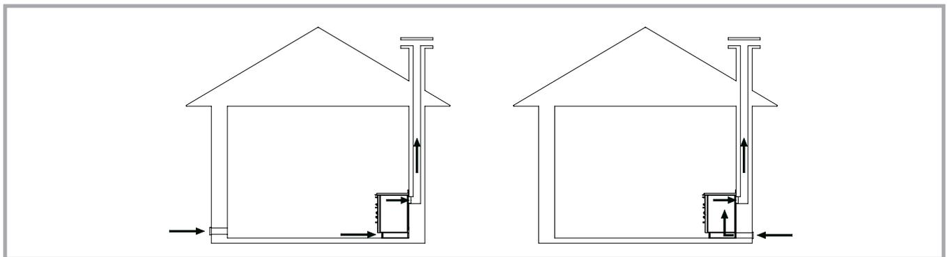
Picture 9 - Installation with air intake in the room and installation with external air intake connected directly to the thermal wood fired cooker.
