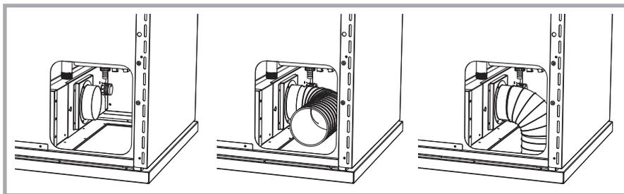
To make the connection easier we suggest to make the external air intake on the floor in correspondence with the internal part of the plinth, or on the wall through the rear part of the thermal cooker (see pictures 11-12). Are also possible other solutions for the connection but they must be decided together with Rizzoli.
