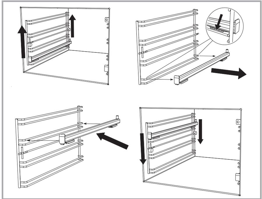
Picture 45 - Instructions for the variation of the position of the telescopic pullout.
