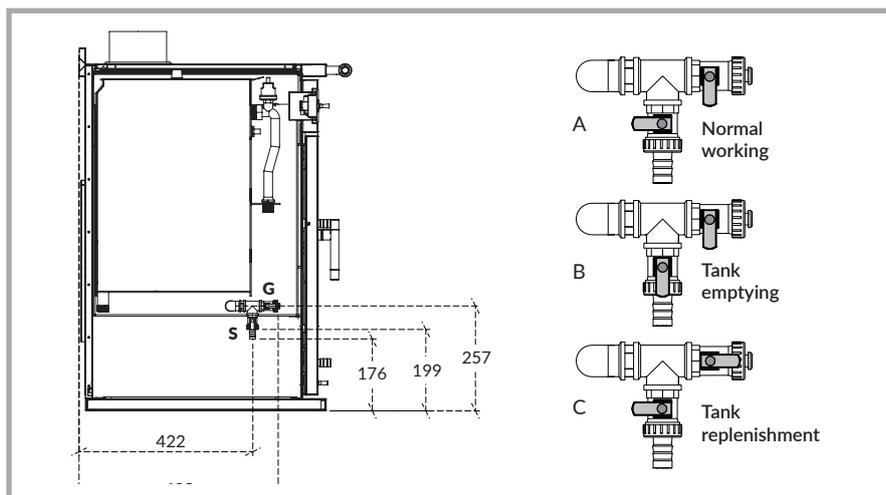
Picture 21 – Connectors for emptying and replenishment of the tank.
