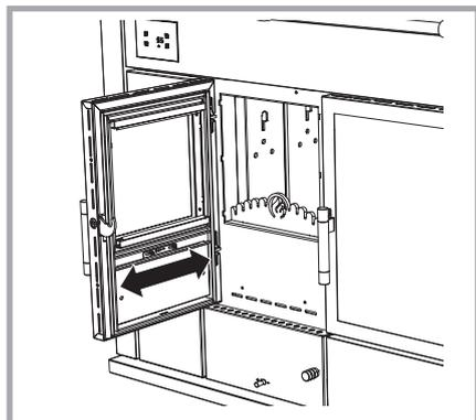
Picture 39 - Air adjustment for glass cleaning.
