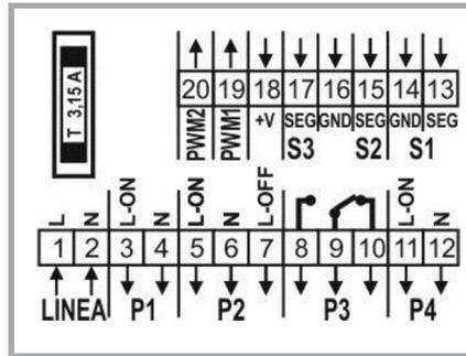
Picture 28 – Electric connections control unit.
