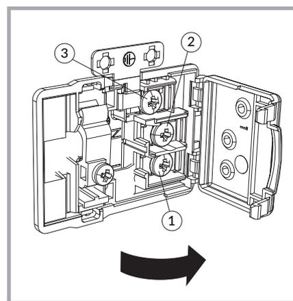
Picture 15 - Terminal board for the connection to the network: 1. Line 2. Neutral 3. Earth.
