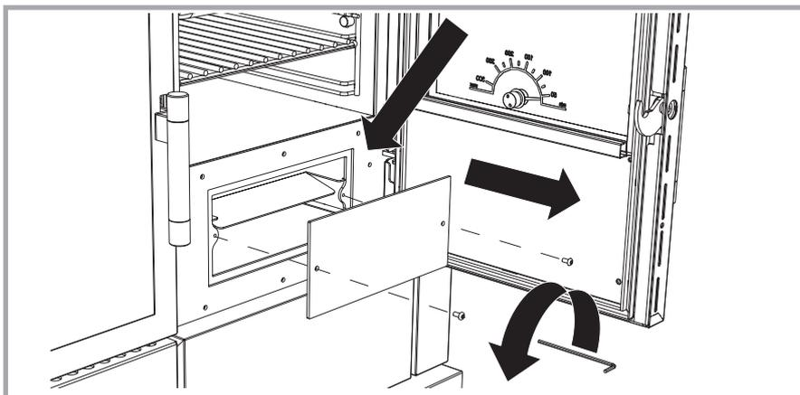
Picture 49 - Fume-circuit inspection.
