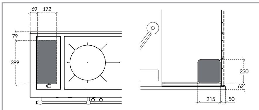
Picture 18 - Position of the lower hole for the passage of the pipes.
