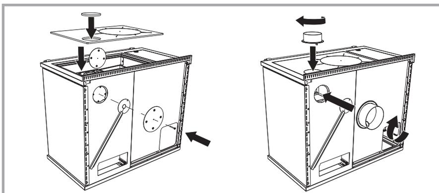
Picture 5 - Predisposition of the flue outlet (STP).
