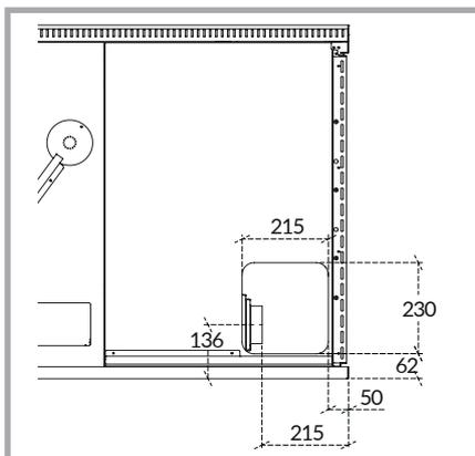
Picture 11 – Position of the rear hole for the passage of the air intake conduct. Dimensions in mm.
