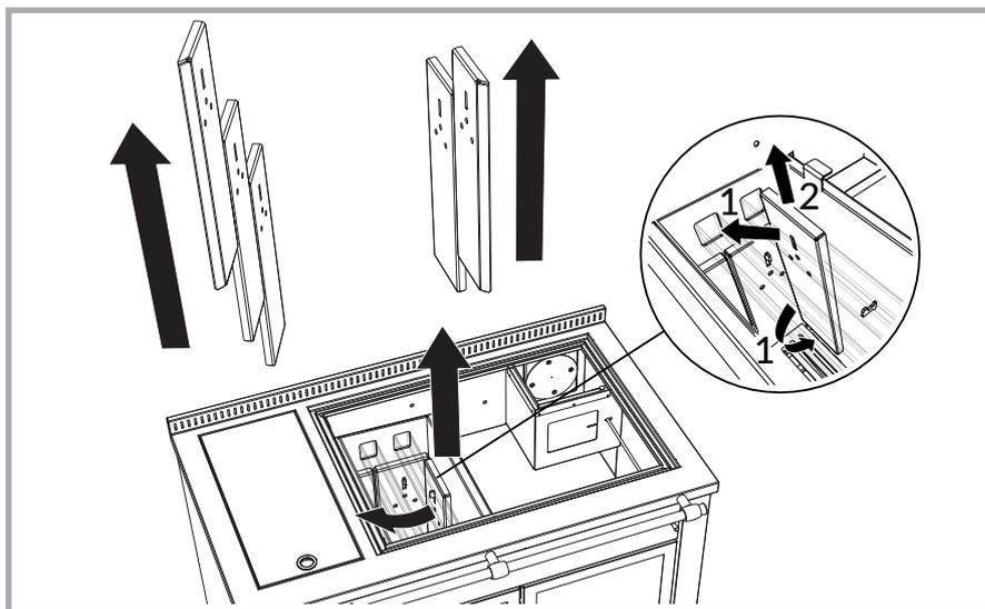
Picture 48 – Maintenance of the combustion chamber sheets.
