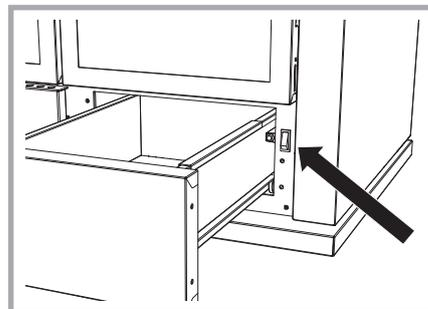
Picture 43 - Switch to light the oven.
