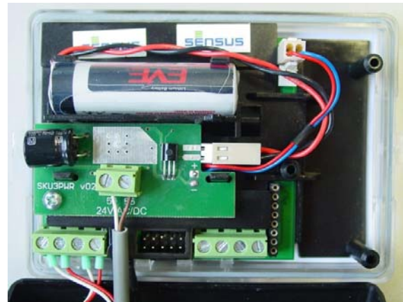
Figure 8: With connected voltage supply
