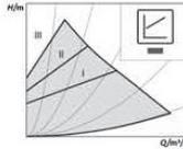
Recommended for two-pipe heating systems with radiators to reduce the flow noises at thermostatic valves.
