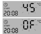
6. Setting STOP zone start time. Icon STOP is lit and hours field is blinking. With arrow keys change active parameter and press Timer button
