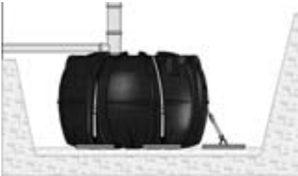
Anchoring with anchor plates.
