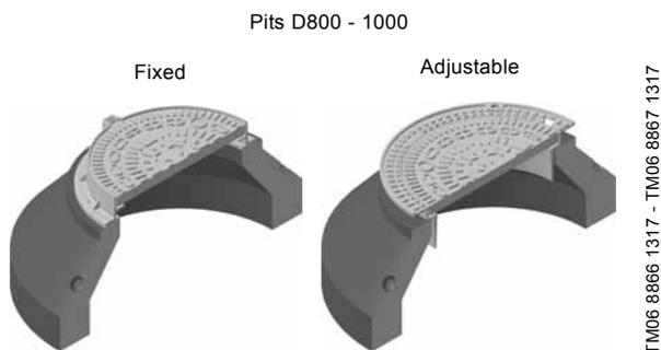
**Fig. 24** Traffic covers for D800 - D1000 pits
