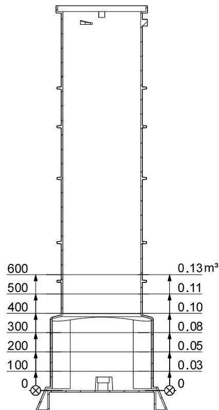
Fig. 37 Effective volume in relation to level, PS.R.05
