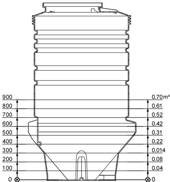
Fig. 40 Effective volume in relation to level, PS.R.12 (one pump)
