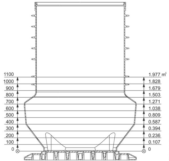
Fig. 42 Effective volume in relation to level, PS.R.17
