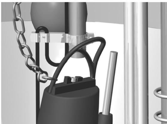
Fig. 34 Chain fitted to pump
