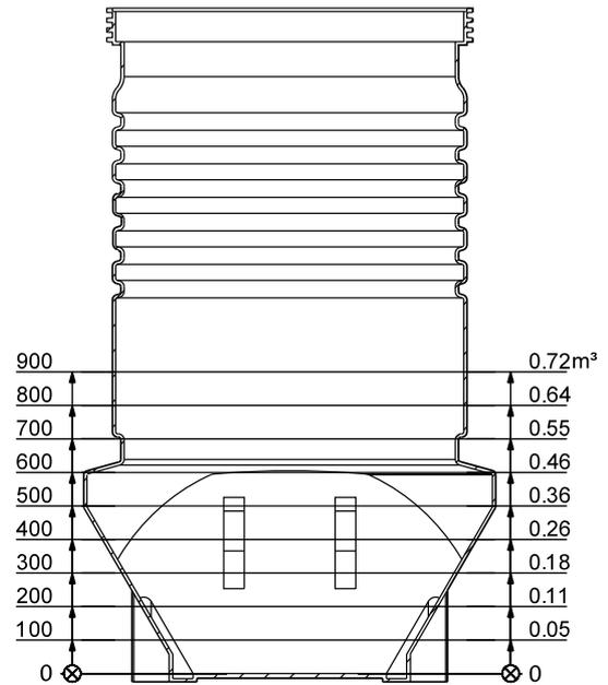
Fig. 41 Effective volume in relation to level, PS.R.12 (two pumps)
