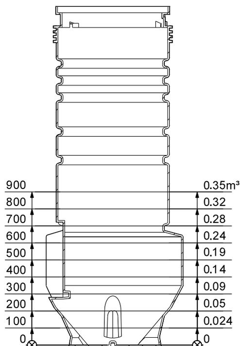
Fig. 38 Effective volume in relation to level, PS.R.08
