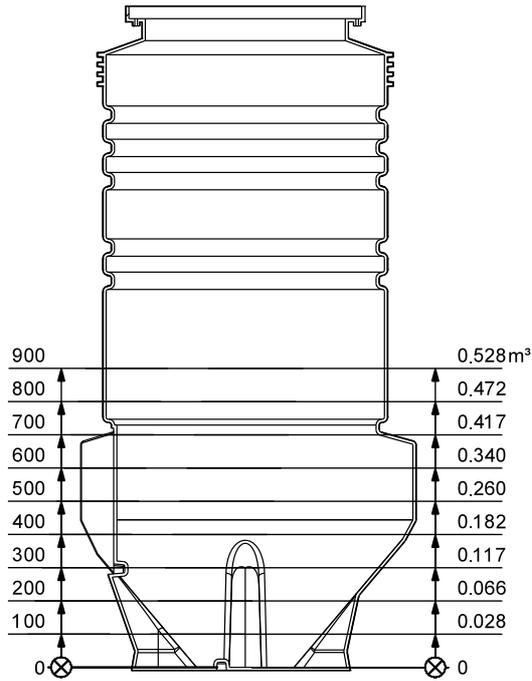
Fig. 39 Effective volume in relation to level, PS.R.10
