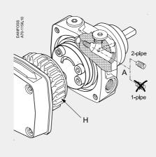
2-pipe: Screw (A) fitted 1-pipe: Screw (A) removed In 2-pipe systems the excess oil is led back to the return outlet (R). In 1-pipe systems with plugged return outlet (R) and removed bypass screw (A), the oil is returned internally to the gear set (see details in below figure). When the pump is stopped the pressure drops and the spring force in the pressure regulator will move the piston until it seats and the oil flow is shut off effectively.
