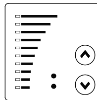
Fig. 17 Control panel of a TPE pump
