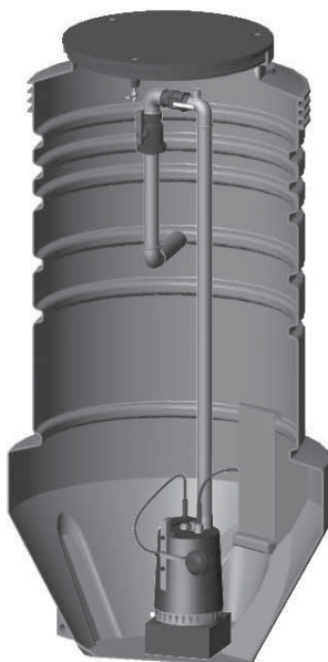
Tank with free-standing pump
