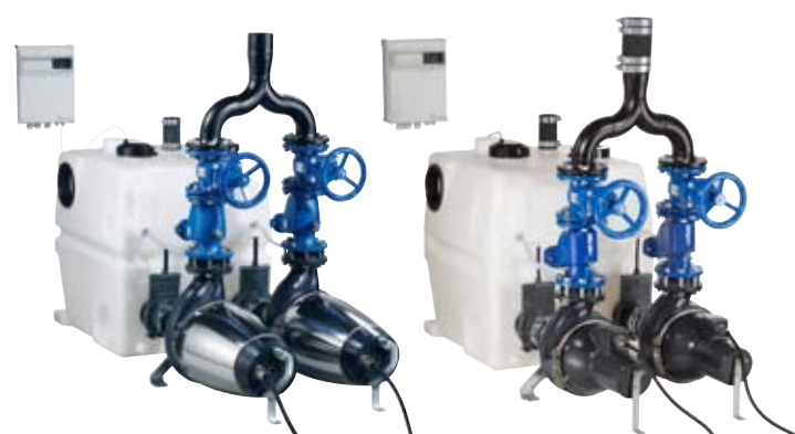
MD1 and MDV stations are fitted with SE1/SEV or SL1/SLV pumps. Container volume from 450 to 1350 l. Max Q: 60 l/s, H: 29 m..
