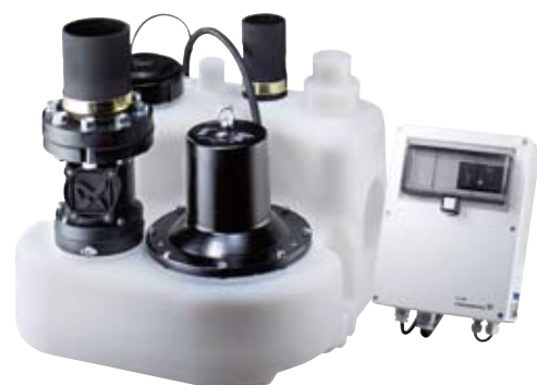
MSS stations have a container volume of 66 l. Max Q: 11 l/s, H: 8.5 m.
