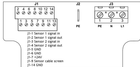
Fig. 7 Connections for power supply / amplifier
