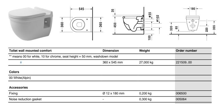
All drawings contain the necessary measurements which are subject to standard tolerances. They are stated in mm and are non-binding. Exact measurements, in particular for customised installation scenarios, can only be taken from the finished ceramic piece.
