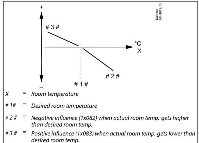
The 'Infl. - max.' and 'Infl. - min.' determine how much the room temperature should influence the desired flow temperature.
