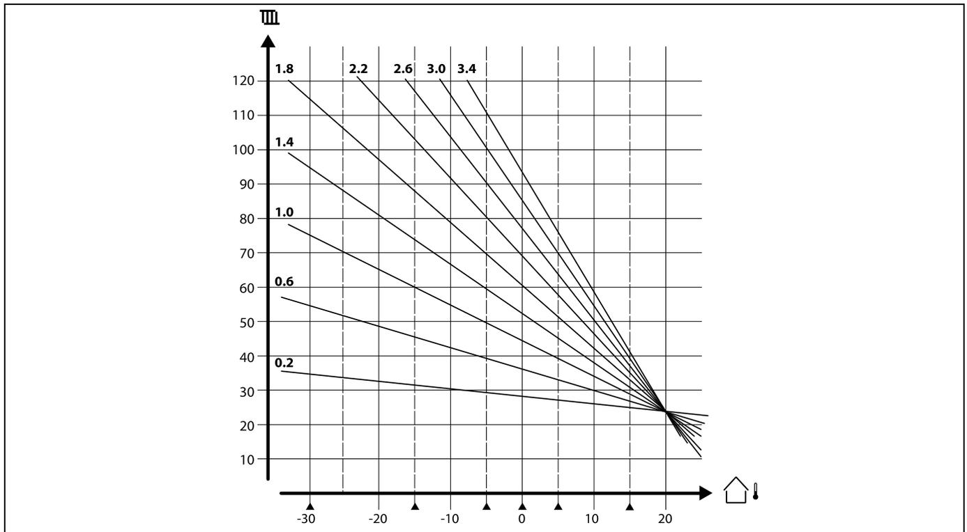
The small arrows (▲) indicate 6 different outdoor temperature values at which you can change the heat curve.
