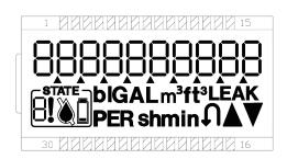
The LCD screen changes automatically to display the following information: net or forward volume, reverse volume, flow rate, events, firmware version, flow direction, meter state.
