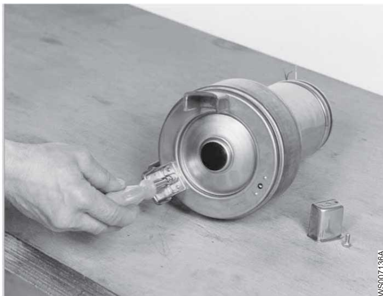
Figure 6: Pump feet removal
