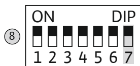
Fig. 16: DIP-brytare 1: intern summer
