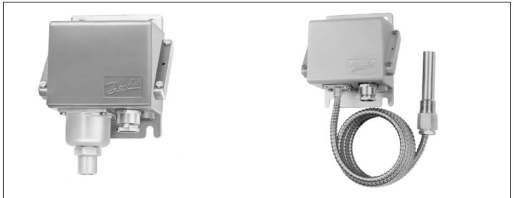
KPS units are pressure-controlled switches. The position of the contacts depends on the pressure in the inlet connection and the set scale value. In this series, special attention has been given to meeting important demands for:
