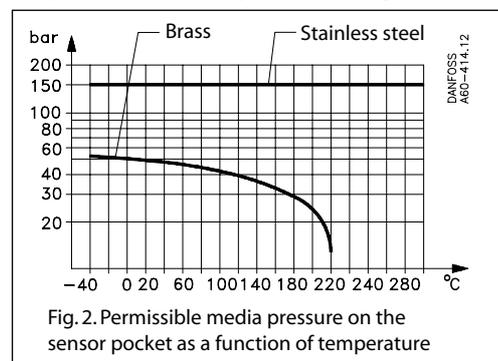
Fig. 2. Permissible media pressure on the sensor pocket as a function of temperature
