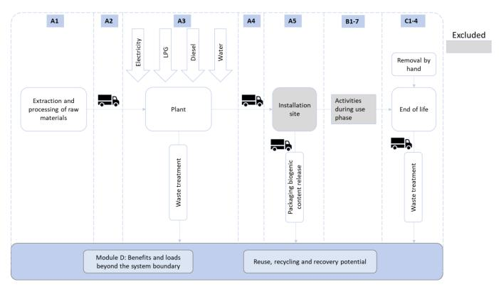
The factory purchases the raw materials and parts from a range of locations across Europe. The transport from suppliers to the Bulgarian factory has been accounted for in A2 and the transport to the Optimera stores in A4.
