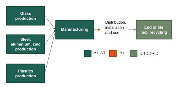
Tempered glass, steel, aluminium, zinc and plastics (polyamide, polyvinylchloride, acrylonitrile butadiene styrene, ethylene-vinyl acetate), are transported to a manufacturing plant where shower enclosures are manufactured. The shower enclosures are transported to a central warehouse from where they are distributed to the final customers. After use the product is transported to waste processing, is manually disassembled and different materials are treated in their respective way.
