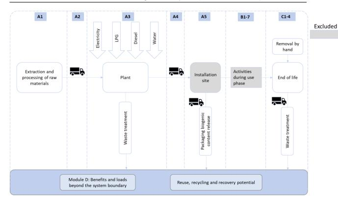
The factory purchases the raw materials and parts from a range of locations across Europe. The transport from suppliers to the Bulgarian factory has been accounted for in A2 and the transport to the Optimera stores in A4.
