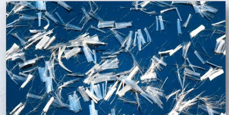
Picture 2: Fibers for concrete
