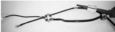
3. Carefully push the antenna cable into the rubber tubing from the side and remove the tool (e.g. screw driver).
