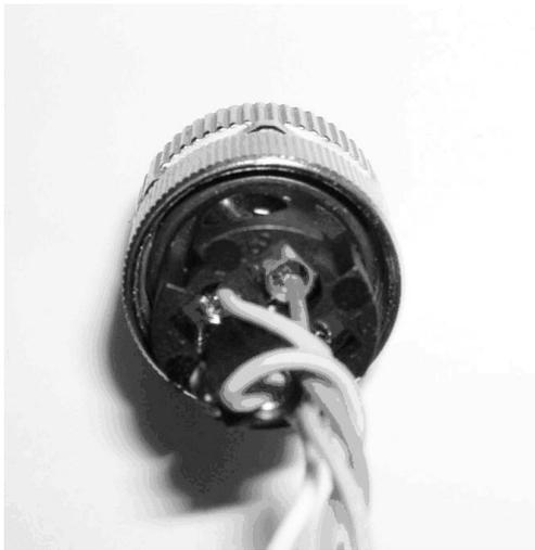
1. Screw together the M12 connector parts, making sure the parts are tightened correctly.
