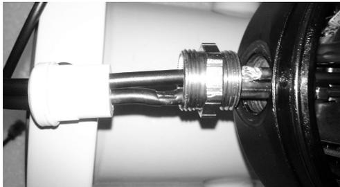
6. Screw M20 cable gland into MAG 8000 housing.
