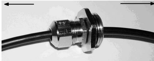
3. Mount M20 to M16 reduction onto the MAG 8000, making sure the reduction is tightened correctly to guarantee IP68 rating.
