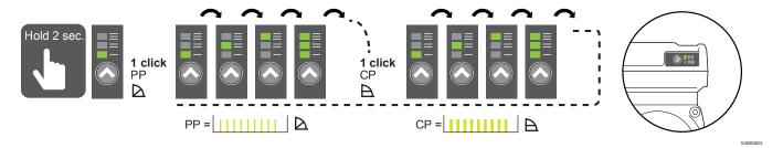
Internally controlled Medium UPM AUTO circulators have a user interface with one pushbutton and three LEDs.
