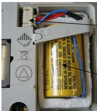
Picture 1: inside view with battery, calculator housing 2
