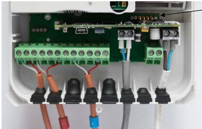
Picture 3: installed option module option module in current version of meter
