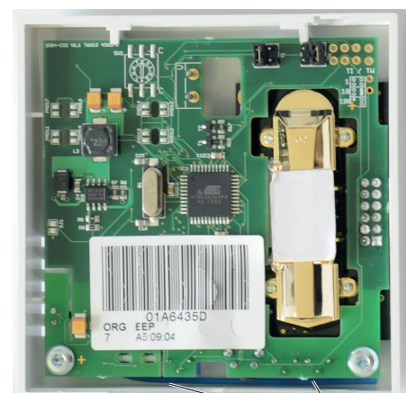
"Learn button"(underneath), to connect to/pair the sensor with Gateway Potentiometers (2) for calibration of rH and CO 2 level respectively
