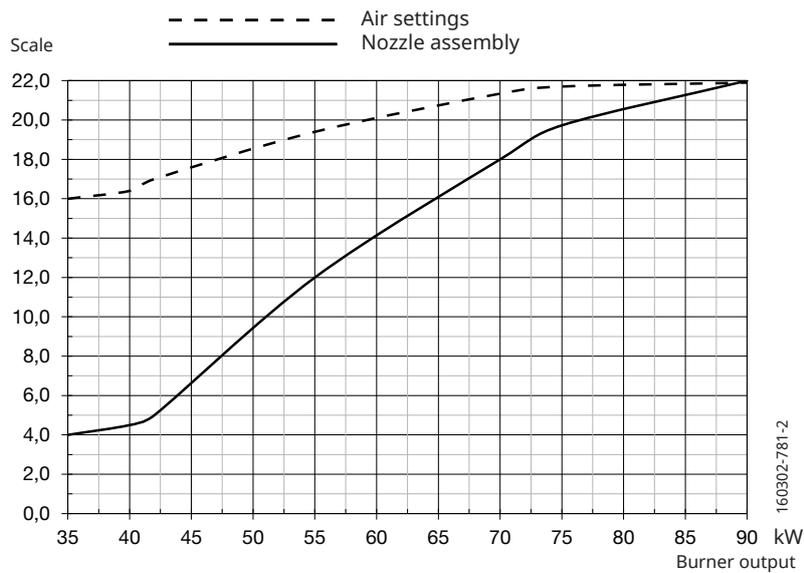
**!** Scale value applies to 0 mbar furnace pressure.
