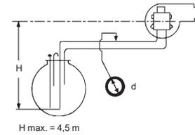
The suction line tables consist of theoretically calculated values where the pipe dimensions and oil velocity have been matched so that tur-bulences will not occur. Such tur-bulences will result in increased pressure losses and in acoustic noise in the pipe system. In addition to drawn copper piping a pipe system usually comprises 4 elbows, a non-return valve, a cut-off valve and an external oil filter.
