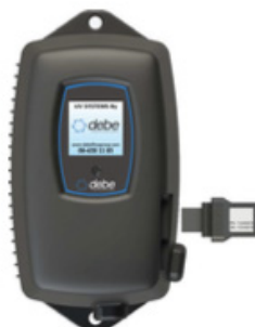
Figure 7. Lamp Key Installation
