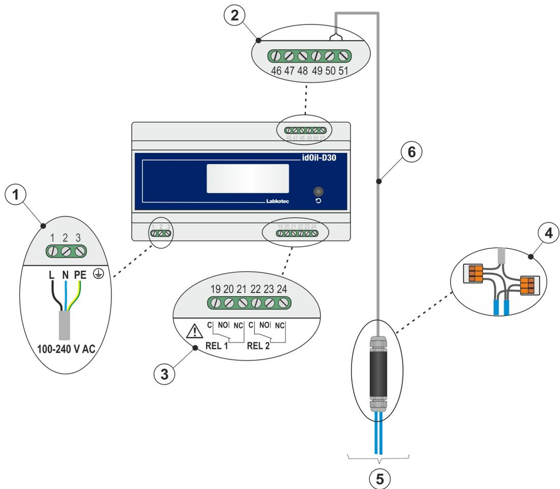
Figure 13. Connection with a two-sensor cable connector
