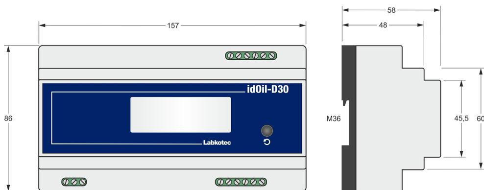
Figure 2. Dimensions of the idOil control unit (mm)
