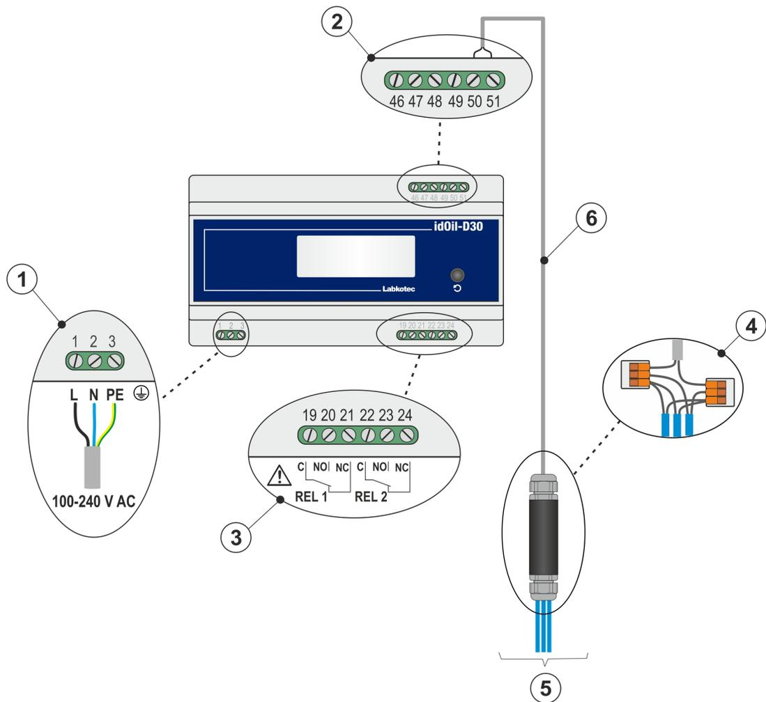
Figure 14. Connection with a three-sensor cable connector
