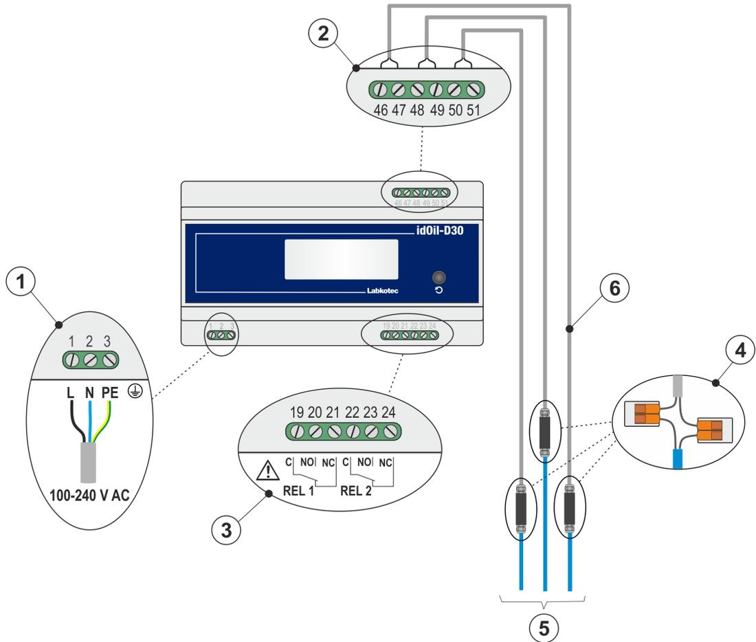
Figure 12. Connection with a single-sensor cable connector
