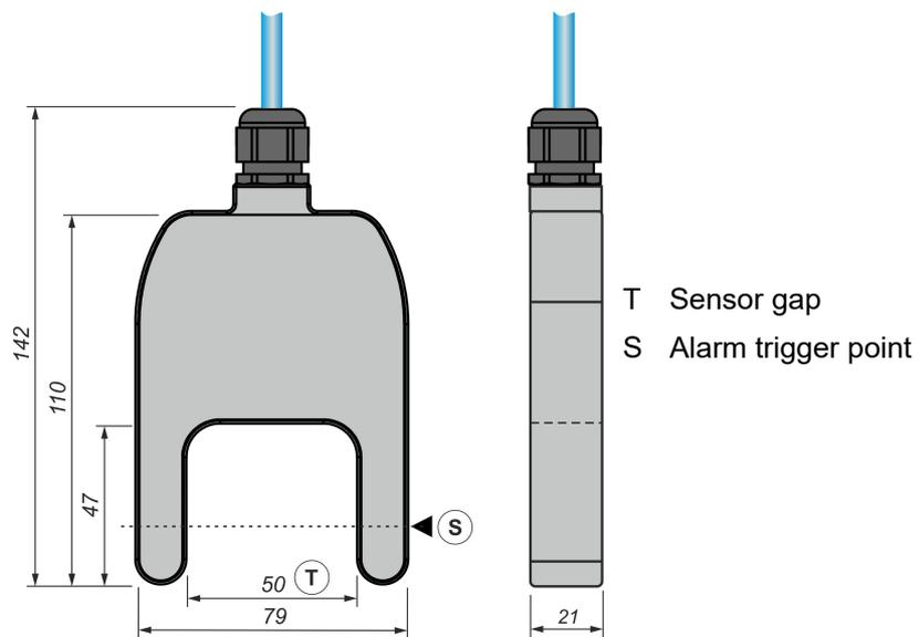
Figure 5. Sludge sensor idOil-SLU – structure and dimensions (mm)
