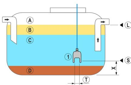
1 idOil-SLU sludge sensor
