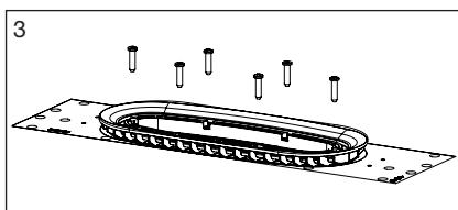
Screw the extension ring into the outlet with the six screws provided.
