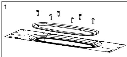
Unscrew the clamping ring from the outlet. Save the screws to the clamping ring. Leave the o-ring in its seat and make sure it is in place.
