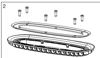
Unscrew the screws in the extension ring and remove the clamping ring. Leave the o-ring in its seat and make sure it is in place.
