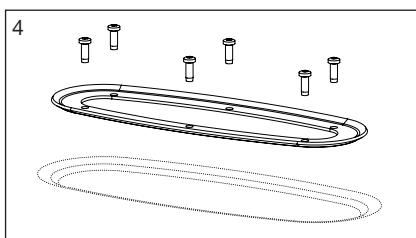
Press down the clamping ring in the seat. In order to facilitate the installation you can make holes with a cylinder in the sleeve for the six screws.
