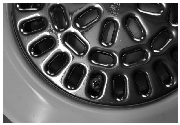
Look thru the grating, there you can see and make sure that the locking clips are fastened under the clamping ring. Take the screwdriver and turn until the grating is in place. A good tip is to screw gently first on one side then the other side, then the first side again. Then you are ready!
