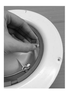
On the locking clip you can see a small flange, this is locking the grating so make sure to get it secured under the clamping ring. Pictures are just to illustrate how they are secured later in the process.
