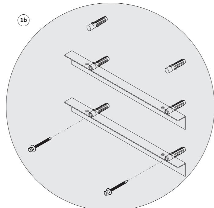
**1a) (GB)** Install the plugs and after that fix the upper bracket.
