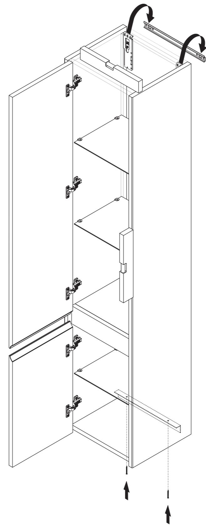
**2) (GB)**Hook the cabinet to the upper bracket and fix it to the lower bracket. Adjust the upper plugs to regulate and tighten the cabinet.
