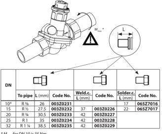
$<sup>*</sup>M_{max}$  for DN 10 is 35 Nm
