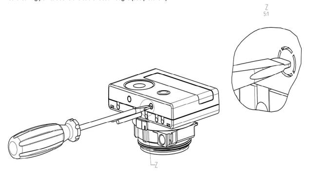
Then insert the screwdriver into one of the two openings at an angle of approx. 45° and carefully lift the handle up to approx. 90° (see picture 2). The upper housing piece of the calculator is then no longer latched on this side. Repeat this with the other opening. Now the upper housing piece can be taken off.
