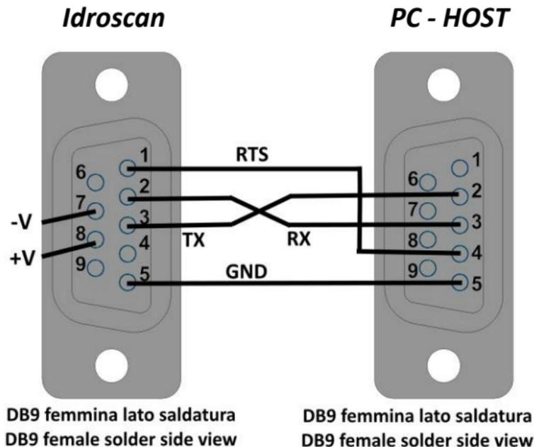
Shielded cable wiring
