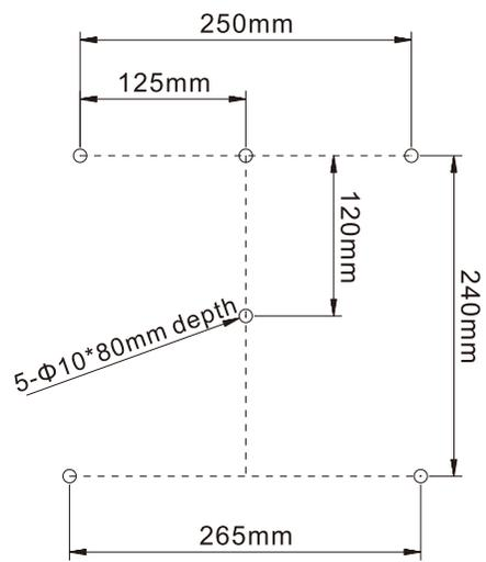
Dimensions for Drilling holes
