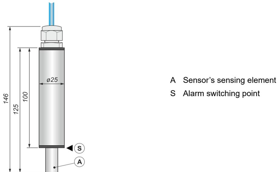
Figure 3. High liquid level sensor idOil-LIQ – structure and dimensions (mm)
