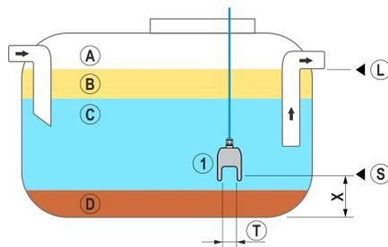
1 idOil-SLU sludge sensor
