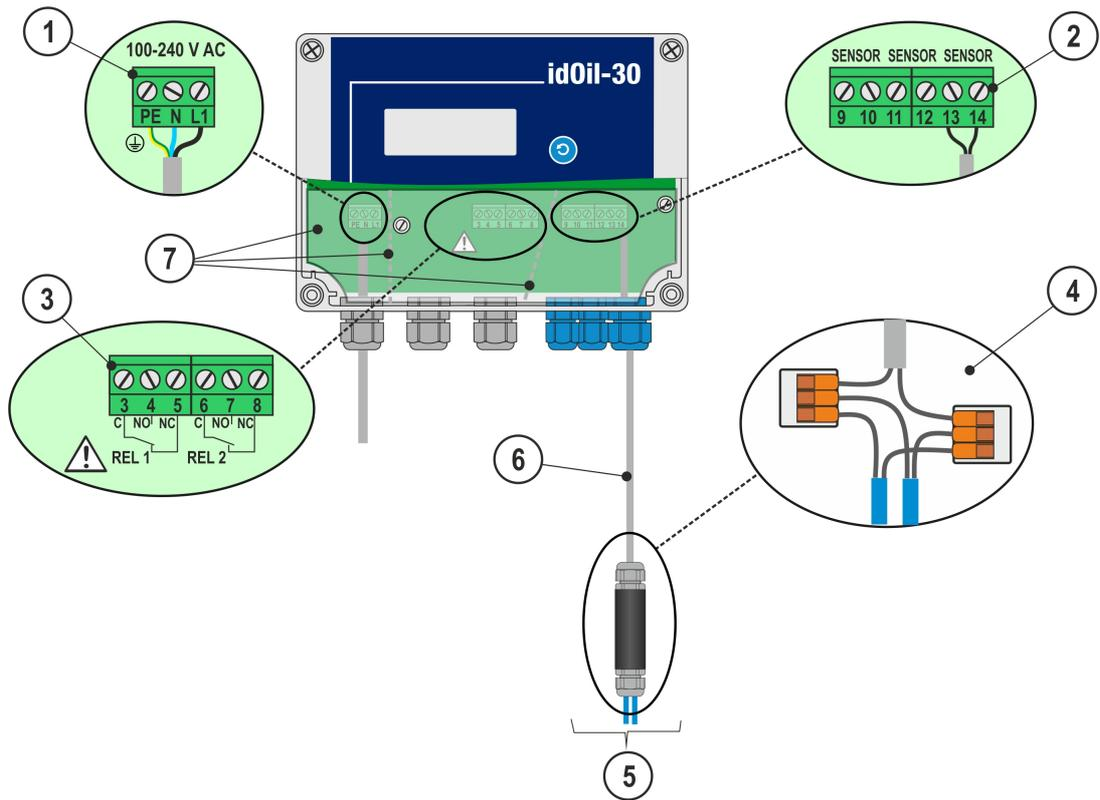
Figure 13. Connection with a two-sensor cable connector
