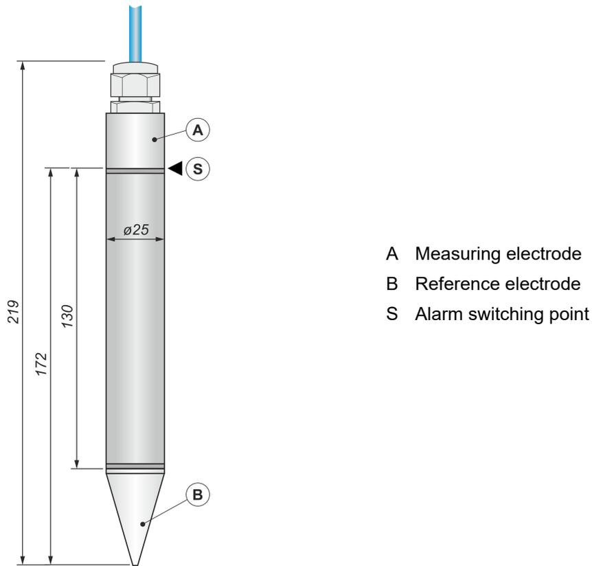
Figure 4. Oil sensor idOil-OIL – structure and dimensions (mm)
