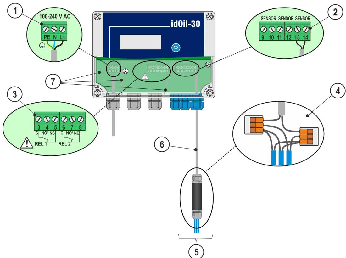
Figure 14. Connection with a three-sensor cable connector
