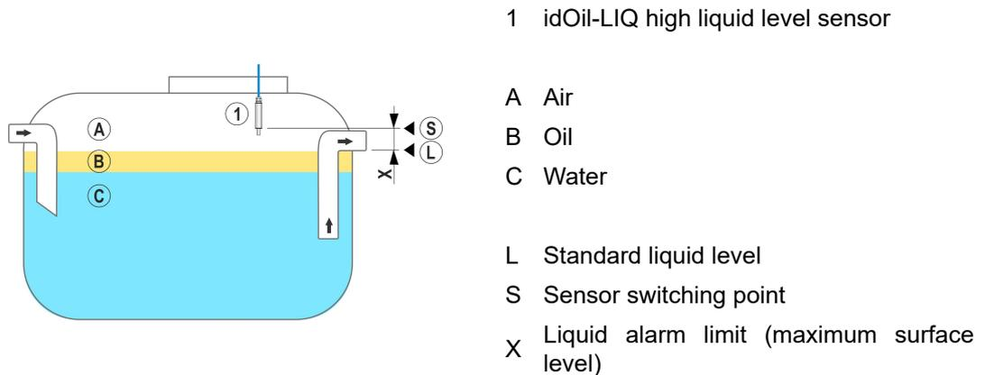
Figure 9. Installing the idOil-LIQ high liquid limit sensor
