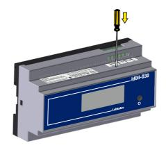
Figure 17. Sensor identification button.
