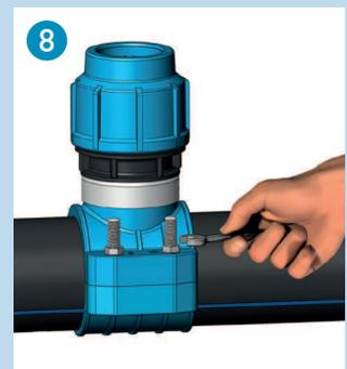
8 Complete the screwing of the bolts until the two parts of the saddle touch each other.
