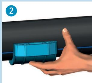
2 Place the bolts in the lower part of the saddle and put it under the pipe.
