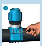
Complete the screwing of the bolts until the two parts of the saddle touch each other.
