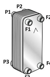
Ports F1/F2/F3/F4 are on the front of the BPHE. Ports P1/P2/P3/P4 are on the back. Note the order in which they appear.
