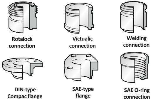
Some connections are equipped with a special plastic cap to protect the connection's threads and sealing surface (X) and to prevent dirt and dust from entering the BPHE. This plastic cap should be removed with care to avoid damaging the thread, sealing surface, or any other part of the connection. Some connections have an external heel whose purpose is to facilitate pressure and leakage testing of the BPHE in production.
