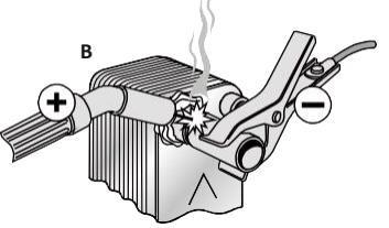
Make sure there are no traces of copper adjacent to the prepared joint. If the joint is prepared by grinding, take appropriate measures to prevent copper from being ground into the stainless surface.
