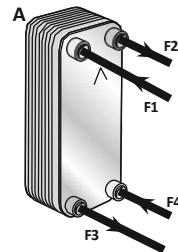
BPHEs with UL approval for use with  $\text{CO}_2$  according to UL files section II or VI. When used with  $\text{CO}_2$ , the system should include a pressure relief valve on each side of the BPHE. The pressure relief valve must open if the system pressure reaches  $0.9 \times$  design pressure.
