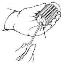
Unscrew the protective cap from the valve body. Remove the central cap covering the adjuster with a small screwdriver.
