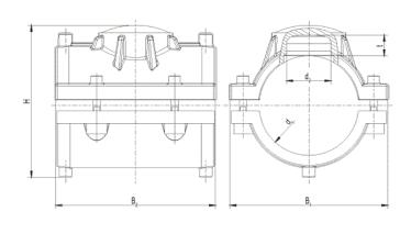
PE 100 SDR 11  ${\it Maximum permissible working pressure 16 bar (water) / 10 bar (gas)}$
